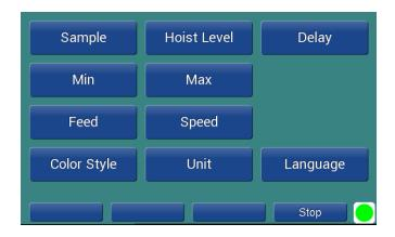
Sample = number of measuring points to be measured (with automatic measurement)
