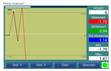
This is the access point for manual measurement. The individual measurement is triggered with Start (or by pressing the foot-operated switch). The display is graphical and numerical. The scaling works as described for the automatic measurement. To return to the main menu, press "Exit".
